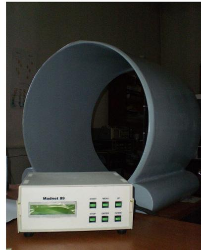
Fig. 6. System for magneto-therapy with "running magnetic field"
