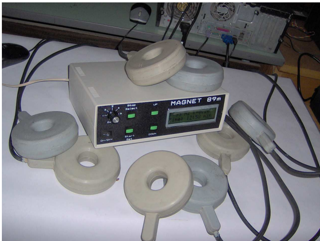
Fig. 2. Apparatus for magneto-therapy with encapsulated inductors
