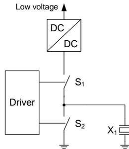
Fig. 2. Pulser circuit
