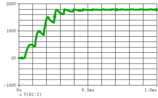
Fig. 4. HV output signal at startup
