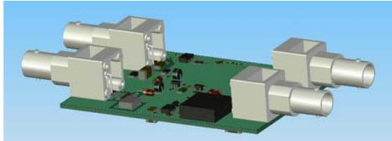
Fig. 7. PCB model in SolidWorks
