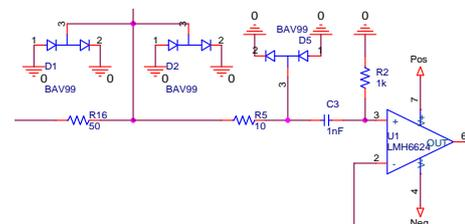
Fig. 6. Input protection circuit
