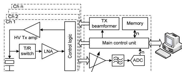
Fig. 1. Simplified system structure
