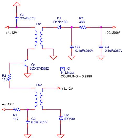
Fig. 3. HV DC-DC converter
