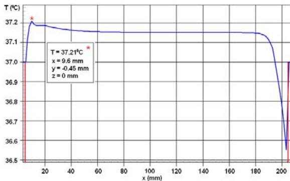
Fig. 2. Temperature in ( $^{\circ}\text{C}$ ) for the case of Figure 1 along the x-axis for  $(y,z) = (-0.45, 0)$  mm. Red vertical lines indicate the sphere diameter
