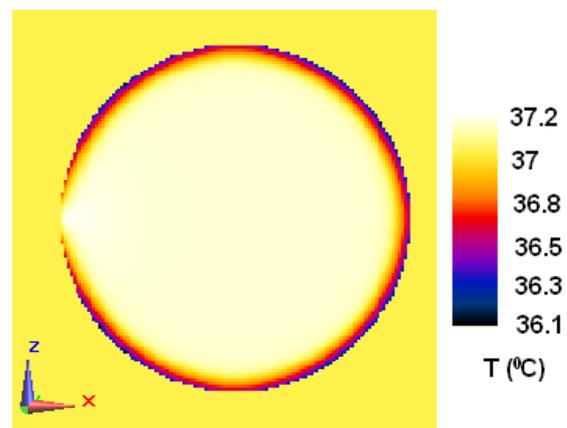
Fig. 1. Temperature distribution in ( $^{\circ}\text{C}$ ) for the case of linear dipole operated at 900 MHz, placed at  $d_1 = 2$  mm, in room temperature of 30 $^{\circ}\text{C}$ . xz plane ( $y = -0.45$  mm) where peak  $\Delta T$  is illustrated.
