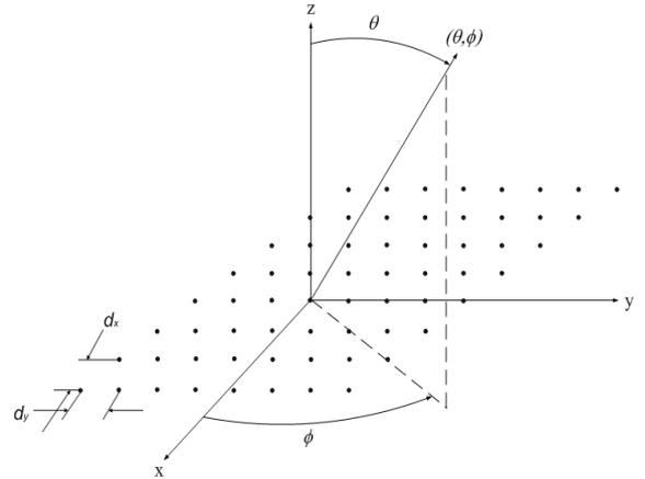
Fig. 3. URA geometry, along with an incoming signal
