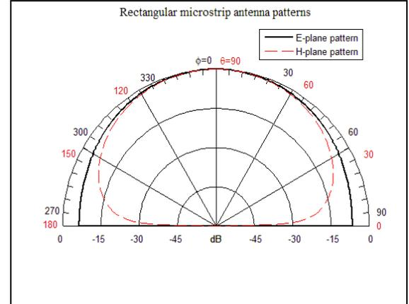
Fig. 4. The rectangular microstrip element radiation pattern
