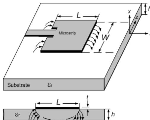
Fig. 1. The rectangular patch element geometry
