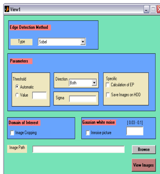
Fig. 1. GUI for edge detection of medical images
