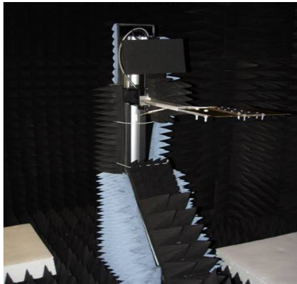
Fig. 1. a) Measurement set-up (transmitter side), b) results obtained by simulation i(black lines) and by measurement (red lines), without operator in the H plane.
