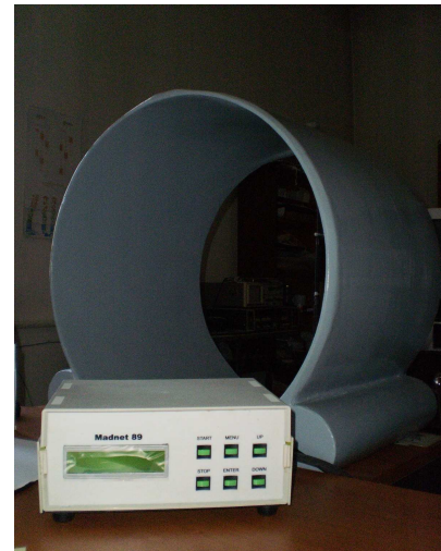
Fig. 6. System for magneto-therapy with "running magnetic field"
