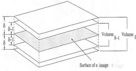
Fig. 1. Volumes of the 'blanket' involved in our proposed algorithm for fractal signature calculation [1]
