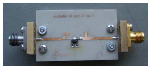
Fig. 4. Test fixture for microwave diode multiplier x5
