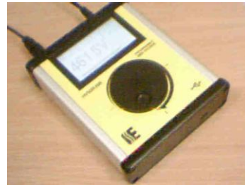
Figure 5. High voltage source photo
