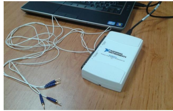
Figure 1. NI USB-6211 DAQ with 4 electrodes
