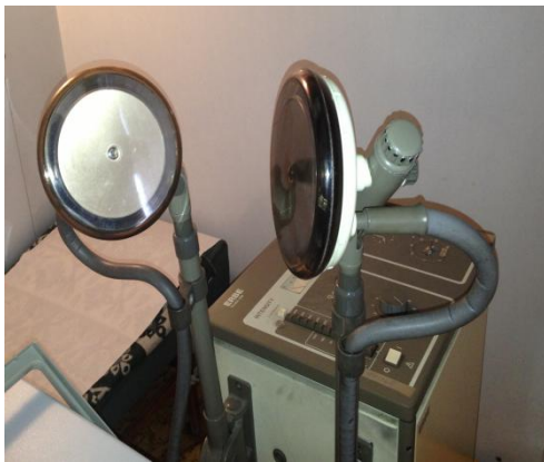
Figure 1. The used antenna system with disc nozzles of each of the emitters during the study of space-time configuration of the electromagnetic field
