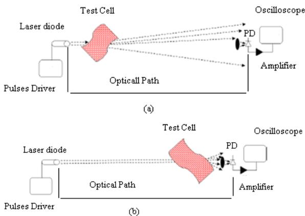
Figure 3. Sketch of diverted beams due to turbulence source positioned (a) near the transmitter and (b) near the receiver
