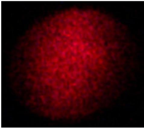
Figure 2. laser spot after passes through the frosted glass
