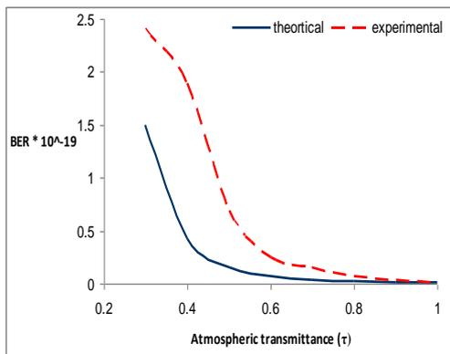
Figure 2. The theoretical and experimental of the BER as a function of atmospheric transmittance
