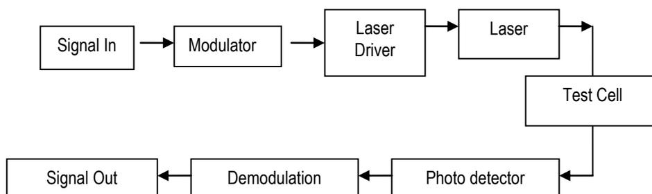
Figure 1. Block diagram of experiment setup
