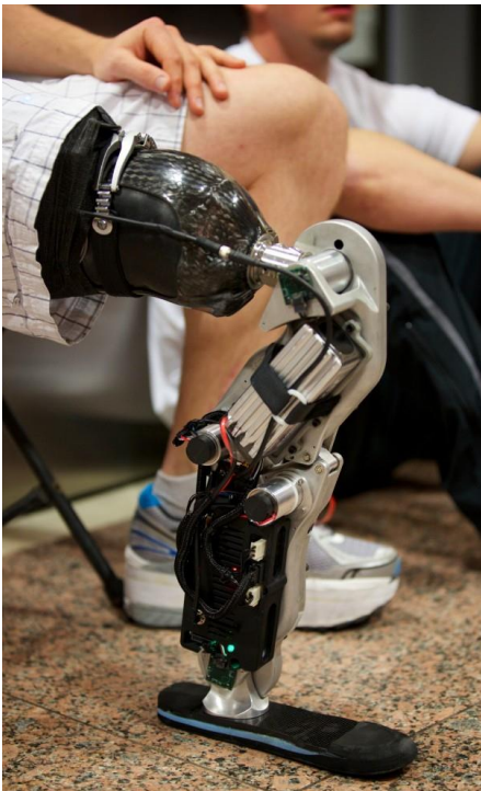
Fig. 5 Rehabilitation Institute of Chicago Bionic leg, used by Zac Vawter to climb 103 floors of Chicago's Willis Tower
