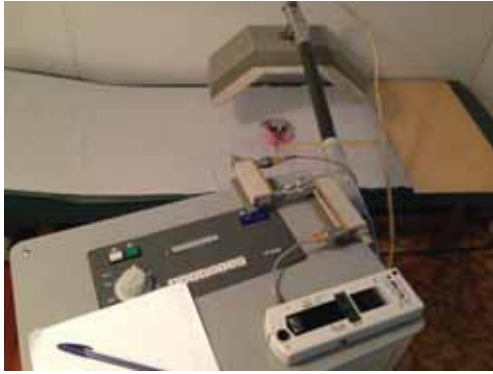
Fig. 2. Setting with symmetric dipole antenna
