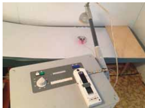
Fig. 1. Setting with asymmetric dipole antenna
