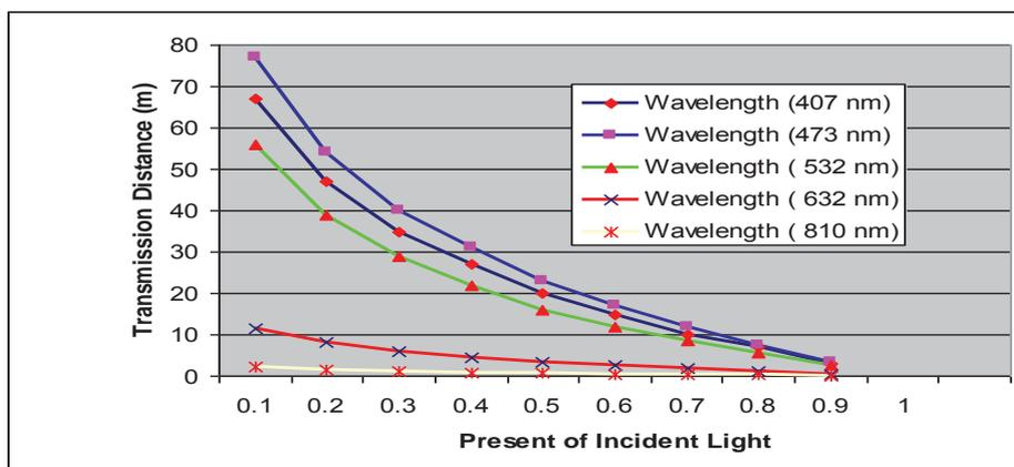
Fig. 5. The transmission Distance for Clear Water at different wavelength of Incident light
