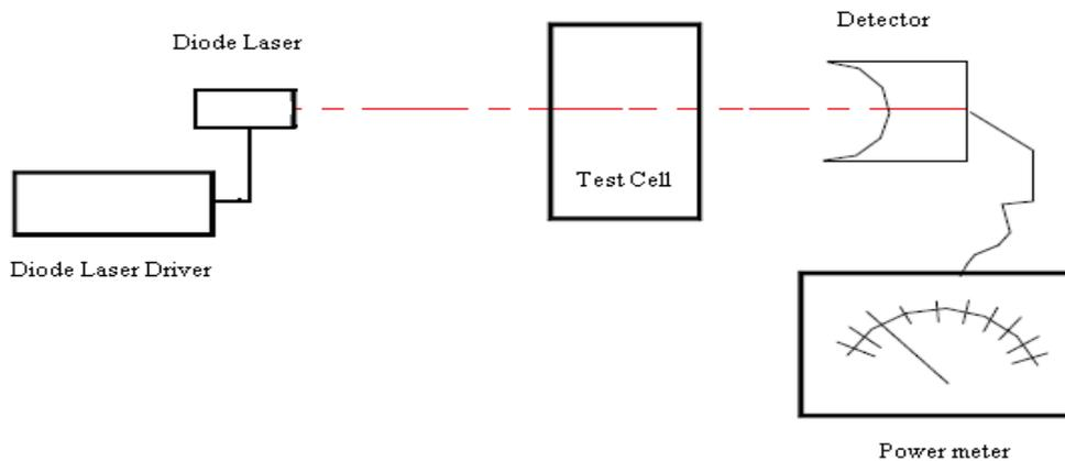
Fig. 2. Schematic set up for measuring absorption coefficient
