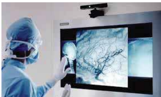
Fig. 1. Kinect-based touchless medical imaging system [12]
