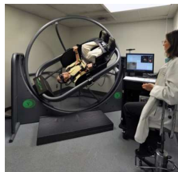
Figure 2: Complex system for vestibular testing
