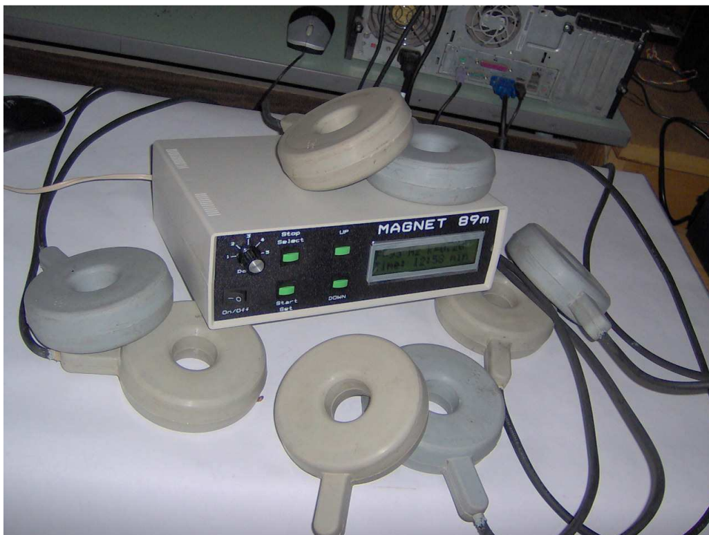
Fig. 2. Apparatus for magneto-therapy with encapsulated inductors
