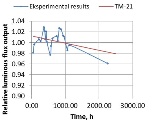
Figure 5. GU10 4X2W (WW) degradation curve
