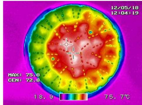
Figure 4. Thermal image of GU10 5050-F24 #1
