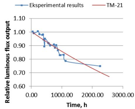
Figure 8. GU10-5050-F24 #2 degradation curve
