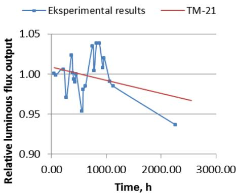
Figure 6. GU10 3X1W-AC-L WW degradation curve
