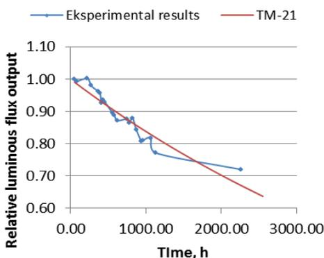
Figure 7. GU10-5050-F24 #1 degradation curve
