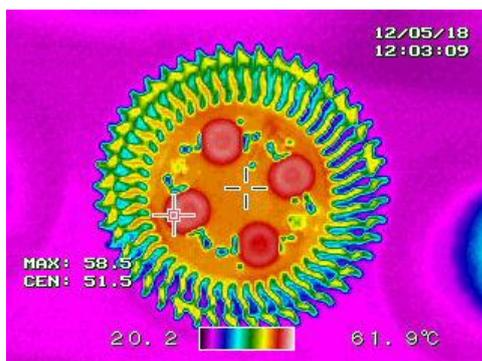
Figure 3. Thermal image of GU10 4X2W-WW
