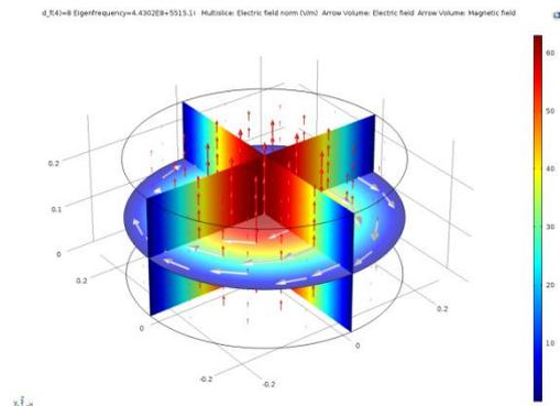
Figure 3. Electromagnetic field distribution inside the resonant cavity
