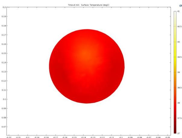
Figure 5. Temperature distribution in liver tissue after 6 minutes of heating
