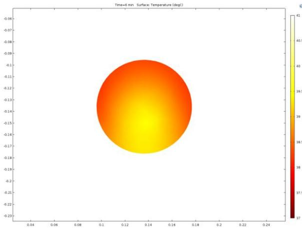
**Figure 9.** Temperature distribution in fat tissue after 6 minutes of heating
