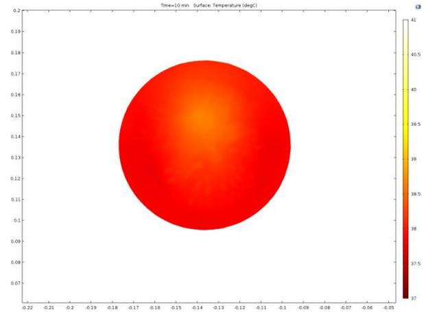
Figure 6. Temperature distribution in liver tissue after 10 minutes of heating
