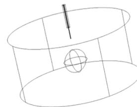
Figure 2. The geometry of the model. The sphere inside the resonator represents the biological tissue.
