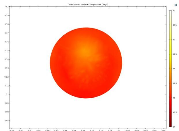
Figure 8. Temperature distribution in muscle tissue after 10 minutes of heating
