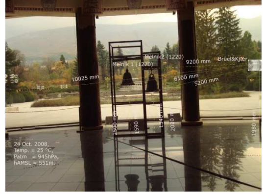
Figure 1. Measuring microphone toward XIII century bell disposition.
