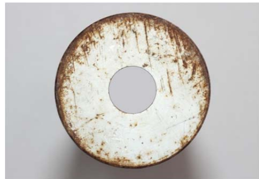
Figure 6. Photograph of the cross-section with corrosion used for calculation with proposed method
