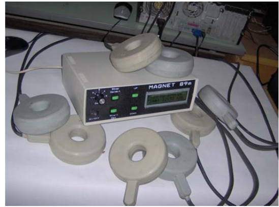
Fig. 2. Electronic unit of system for magneto-therapy together with local inductors
