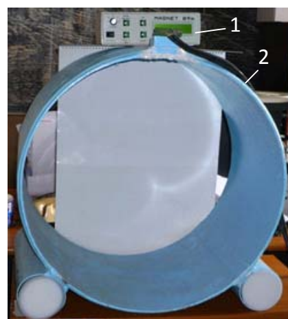
Fig. 5. Girdle coil with "movement" of low frequency magnetic field on the coil's axis
