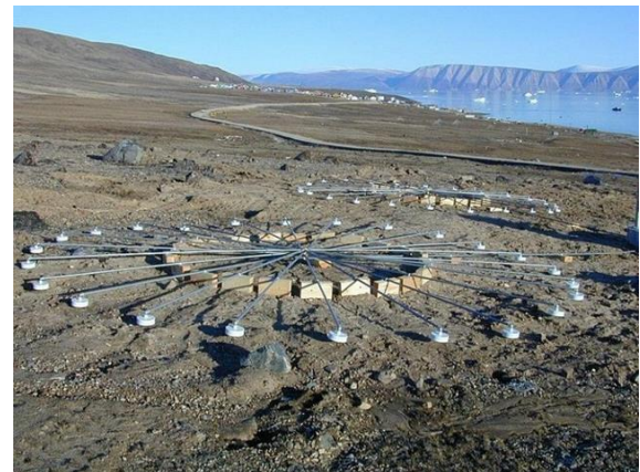
Fig. 2. Acoustic group from infrasound station IS18 in Greenland [1]
