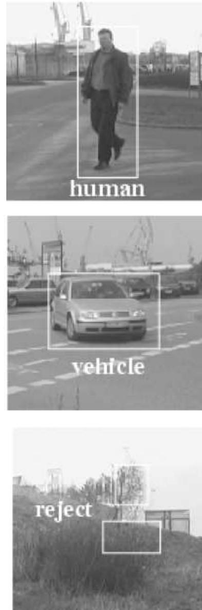
Fig.3. The separated human, vehicle and rejected false moving objects
