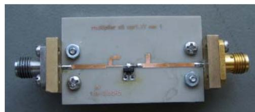
Fig. 4. Test fixture for microwave diode multiplier x5
