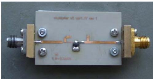
Fig. 6. Diode frequency multiplier with added solder drop between grounded pins
