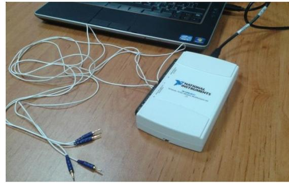
Figure 1. NI USB-6211 DAQ with 4 electrodes
