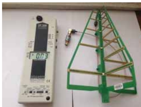
Fig. 3. The metering device and antenna
