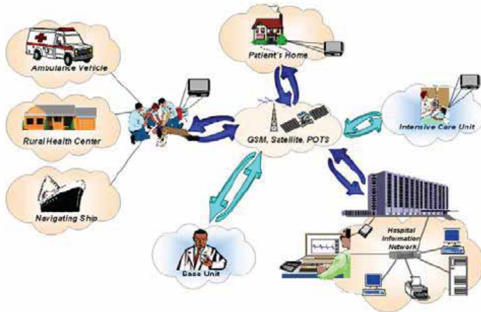
Fig. 1. Communication system for telemedicine
