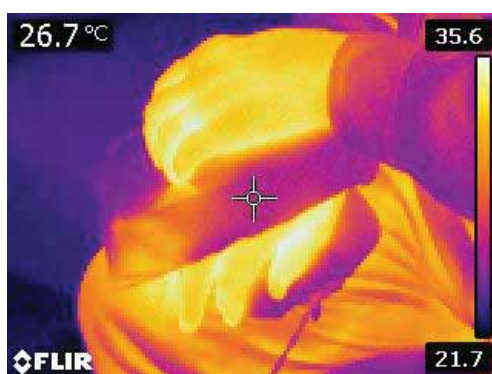
Fig. 3. Infrared image with the measurement of coil temperature
