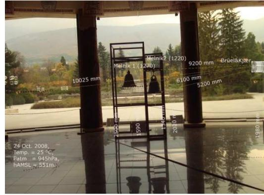
Figure 1. Measuring microphone toward XIII century bell disposition.
