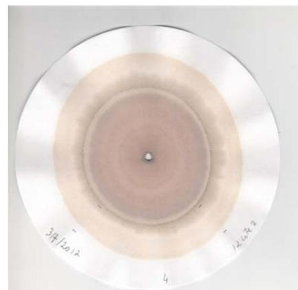
Figure 1. Image of soil sample obtained by the capillary dynamolysis method
