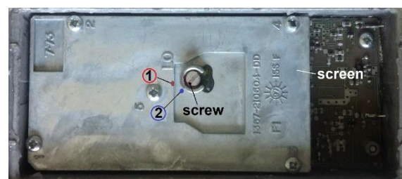
Figure 7. LNB inside (Low subband)
