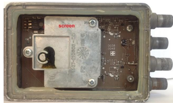
Figure 5. LNB inside (high subband)
