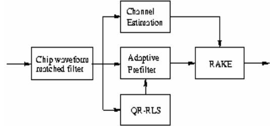
Fig. 2. Prefilter-Rake equalizer
