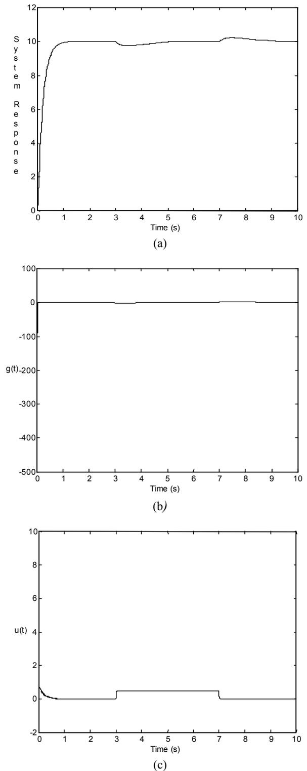
Fig. 2 The system response and the disturbance elimination (a), the switching function response  $g(t)$  (b) and the control  $u(t)$  (c). (the case with the disturbance acting on the plant input)
