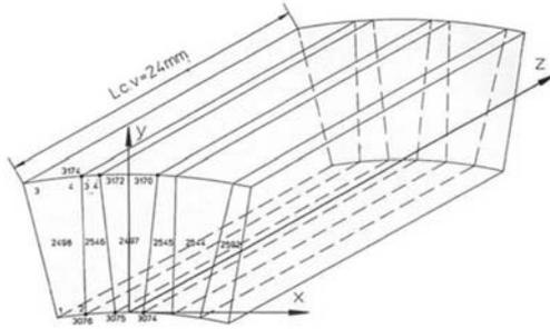
Fig. 4. Local coordinate system in fourth axial layer.  $l_{sIVc.v}=24$  mm – axial length of fourth layer;  $b_k=55.9$  mm – channel width;  $t_1=99.7$  mm pitch channel-tooth;  $b_z=43.8$  mm – width of stator tooth;  $N_k$  – number of conductors per channel
