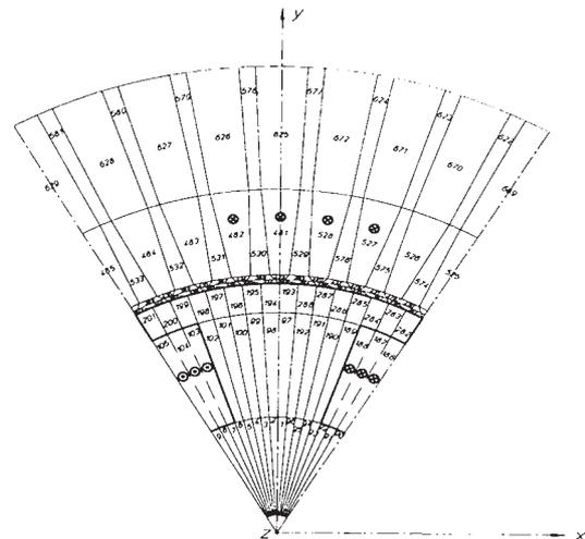
Fig. 1. Cross section of first axial layer with current densities
