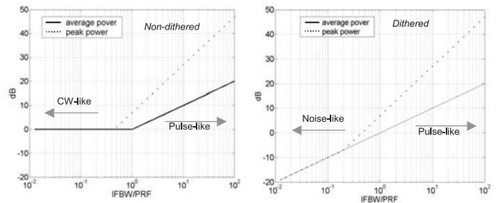
Fig. 2. UWB power at the receiver's IF output
