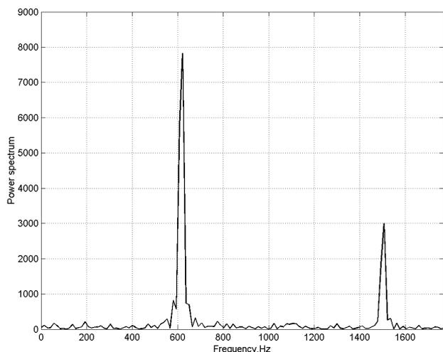
Figure 1 – Spectrum analysis at the frequencies below half the virtual sampling frequency
