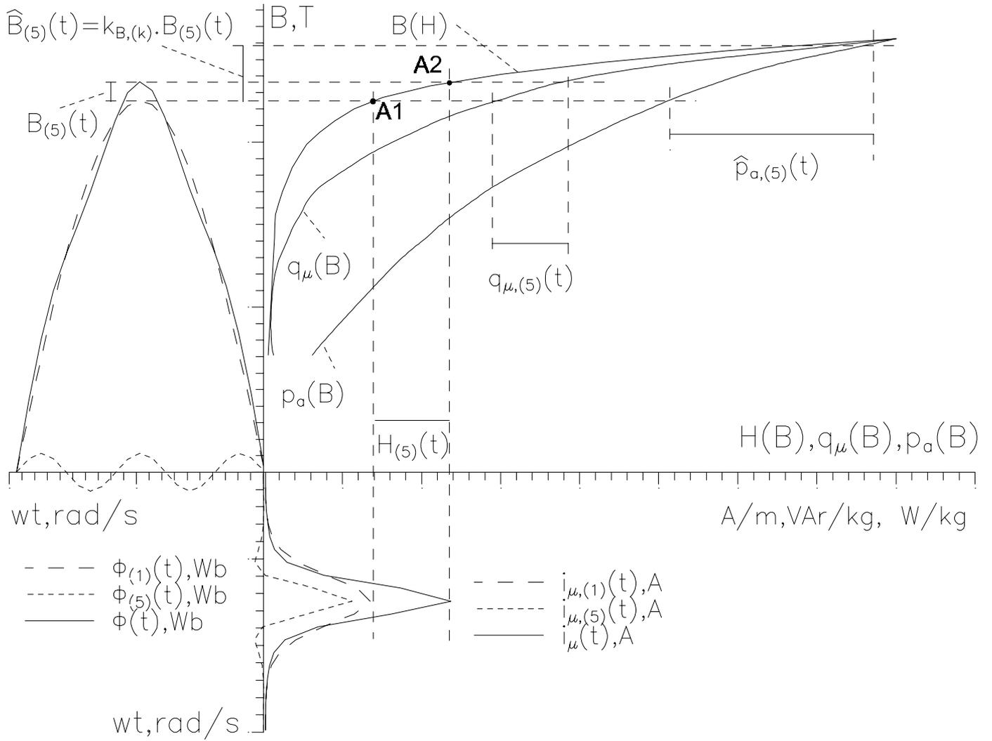
Fig.3. Determining the additional core losses of the transformer for the 5<sup>n</sup> harmonic
