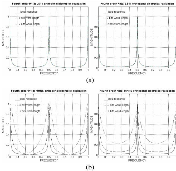
Fig. 3. Magnitude responses of the first-order bicomplex orthogonal sections for different word-lengths: (a) LS11-based for  $\beta=0.01$ ; (b) MHNS-based for  $\alpha=0.99$
