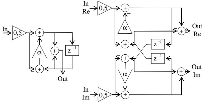
Fig.1. (a) First-order LP MHNS-prototype real sections; (b) MHNS-based orthogonal BP complex section
