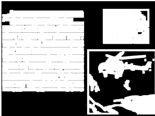
Fig. 8. After dilation for connected component analysis
