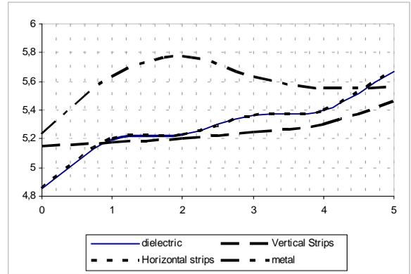
Fig. 6 Gain versus the width  $w$  [mm]
