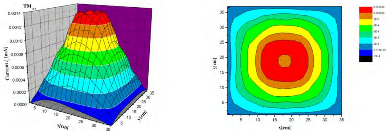
Fig. 5. Induced current for  $TM_{110}$  mode, for probe length  $d=6\text{cm}$
