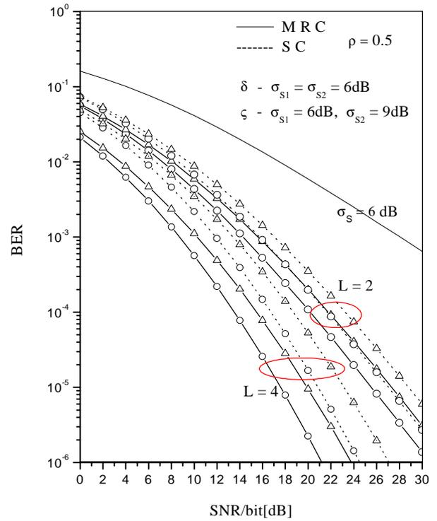
Fig. 4 Dependence of the BER of the SNR/bit for the diversity system with SC and MRC combined micro branches with equal and unequal power in correlated macro branches ( $\rho = 0.5$ ).
