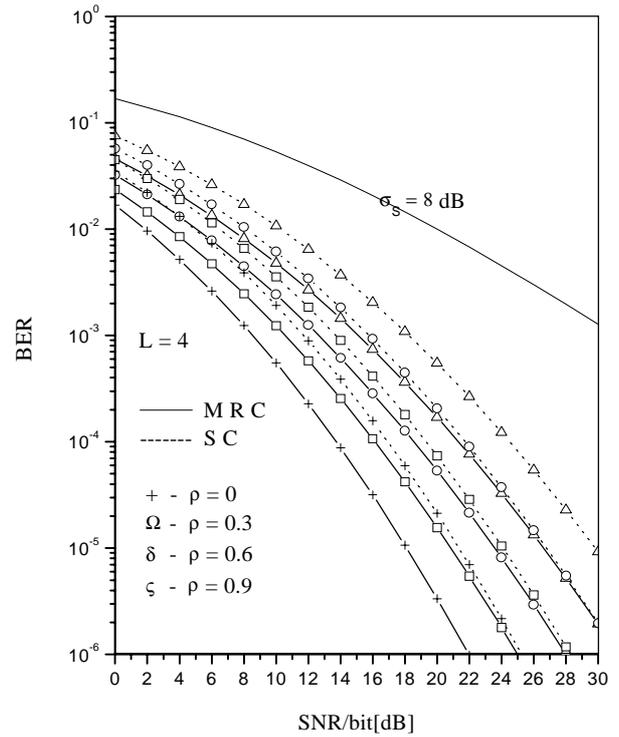
Fig. 2 Dependence of the BER of the SNR/bit for the diversity system with  $L=4$  SC and MRC combined micro branches with different values of correlation coefficient.
