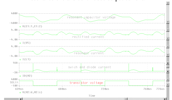
Fig. 13. PSPICE simulation results at a frequency lower than the resonance one and discontinuous output current.
