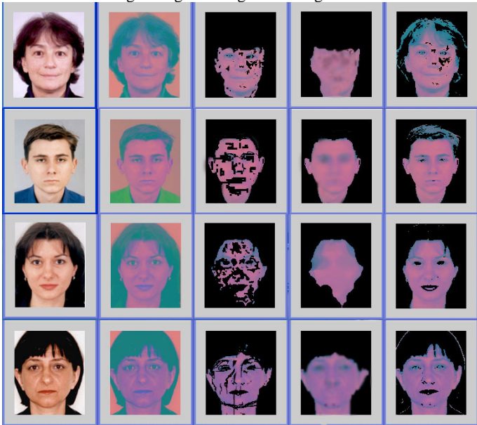
Fig. 4 Original images (RGB), Original images (YCrCb), Mask without smoothing, Mask after morphological filtering, Mask with smoothing;
