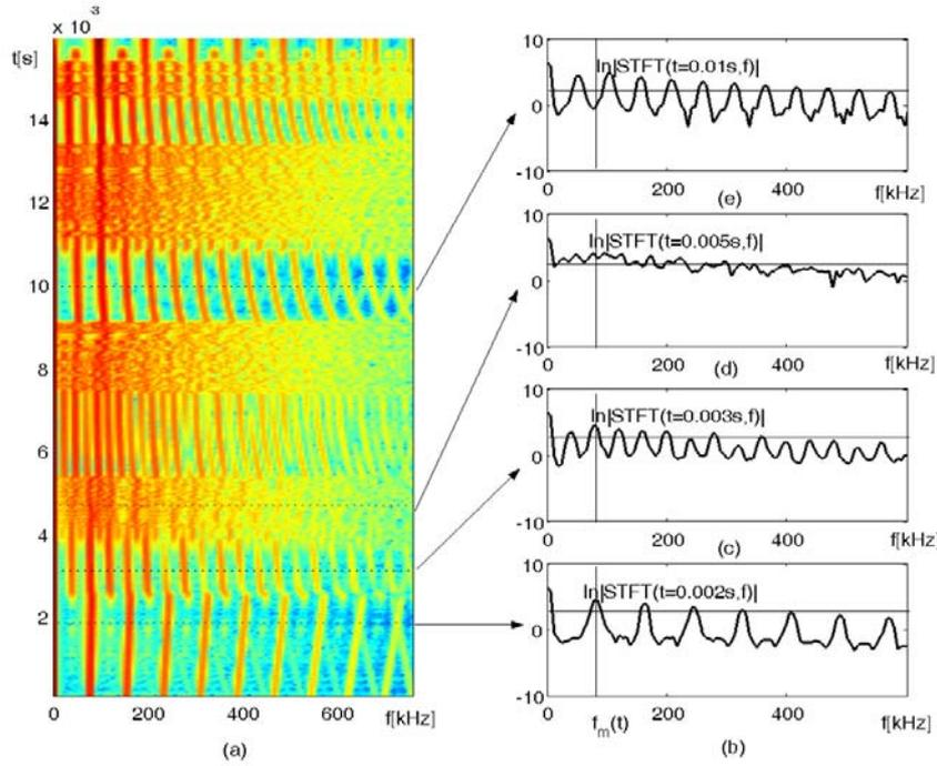
Fig. 3. (a) STFT. (b) Logarithm of the STFT for  $t=2\text{ms}$  - period 1 orbit. (c) Logarithm of the STFT for  $t=3\text{ms}$  - period 2 orbit. (d) Logarithm of the STFT for  $t=5\text{ms}$  - chaos. (e) Logarithm of the STFT for  $t=10\text{ms}$  - periodic window.
