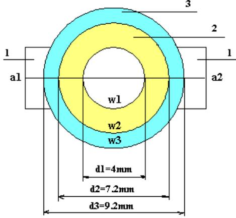
Fig. 1. Example of the cross-section of a discharge device:
