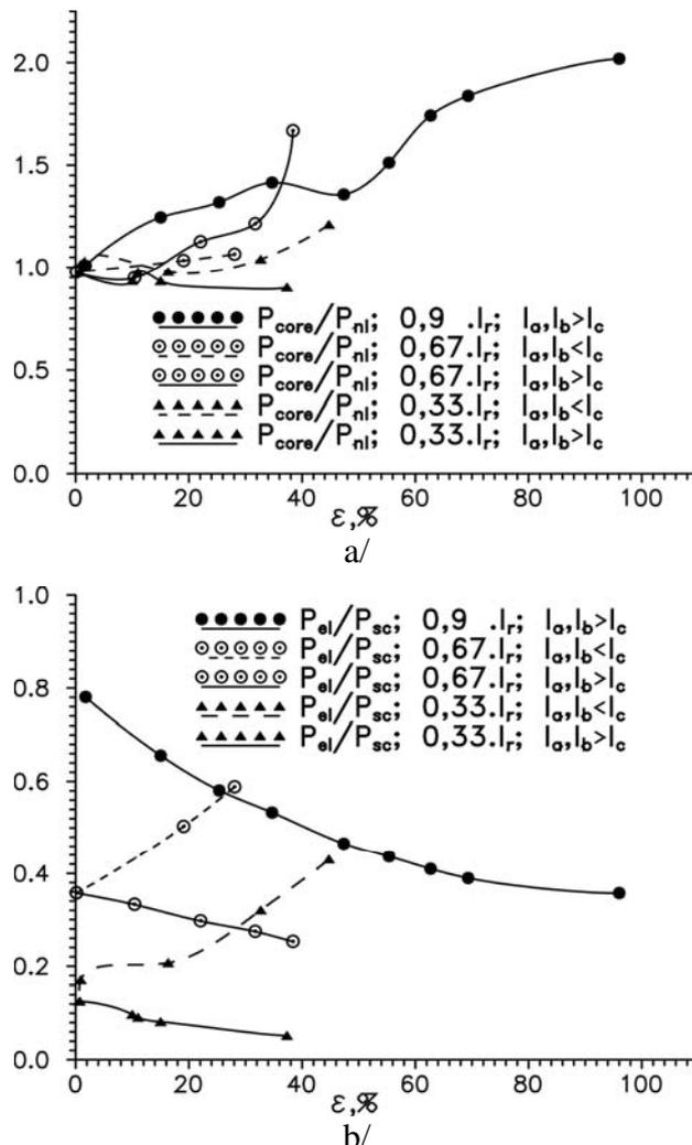
Fig. 10. Transformer losses versus current non-symmetry coefficient
