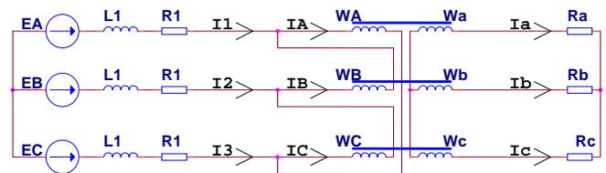
Fig.1 Equivalent circuit
