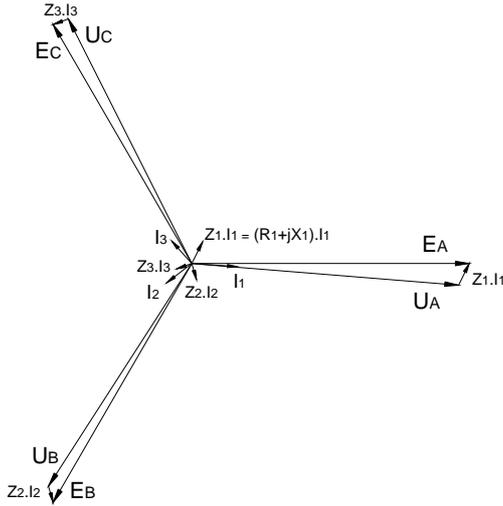
Fig. 3. Phasor diagram of the transformer's supply voltage
