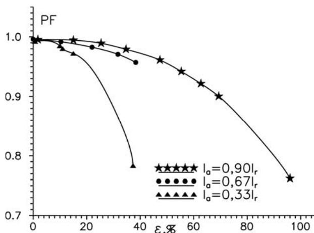
Fig. 9. Power factor versus current non-symmetry coefficient
